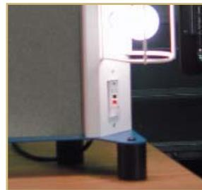
A rocker switch and single grounded outlet are mounted on the mirror surround.
